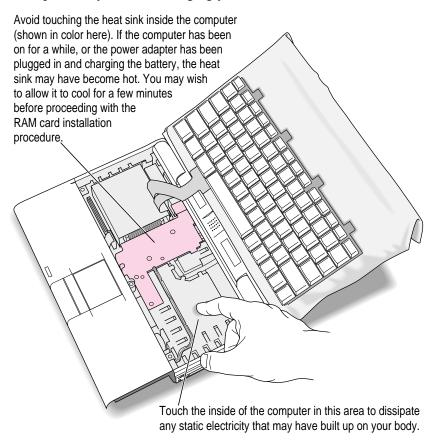
Don't walk around while installing the card. If you do, make sure you do this step again to discharge any static electricity.
